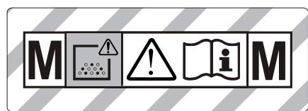
**WARNING:** This unit contains hazardous dust. Emptying and maintenance, including the removal of the dust bag, may only be carried out by someone who is familiar with the unit and wearing suitable protective gear. Do not switch on the unit until the complete filter system has been installed and the function of the volume-flow control has been tested.
